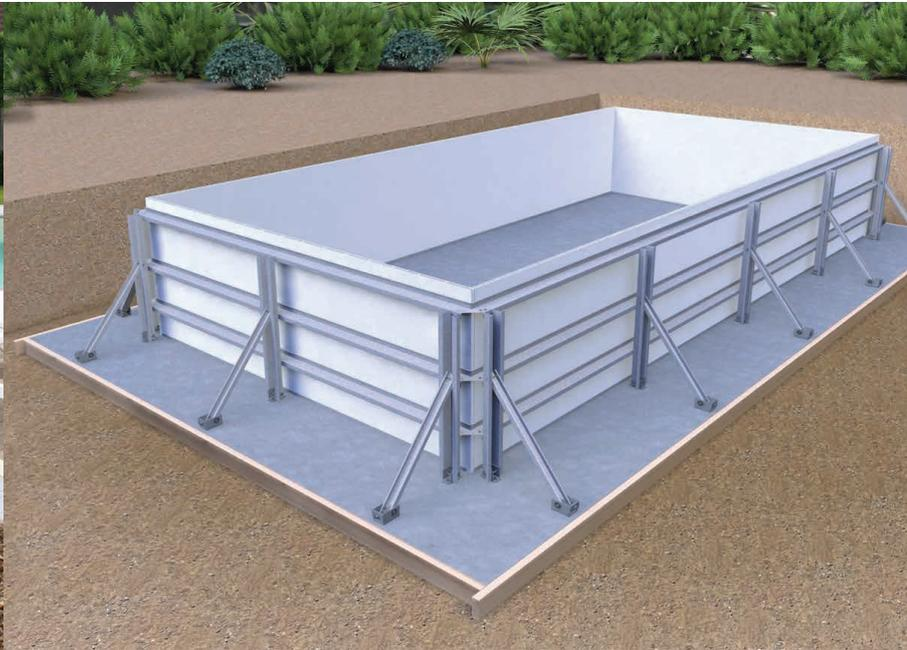
Pool-structure in galvanized steel with walls in pvc strenghtened with glassfibre
